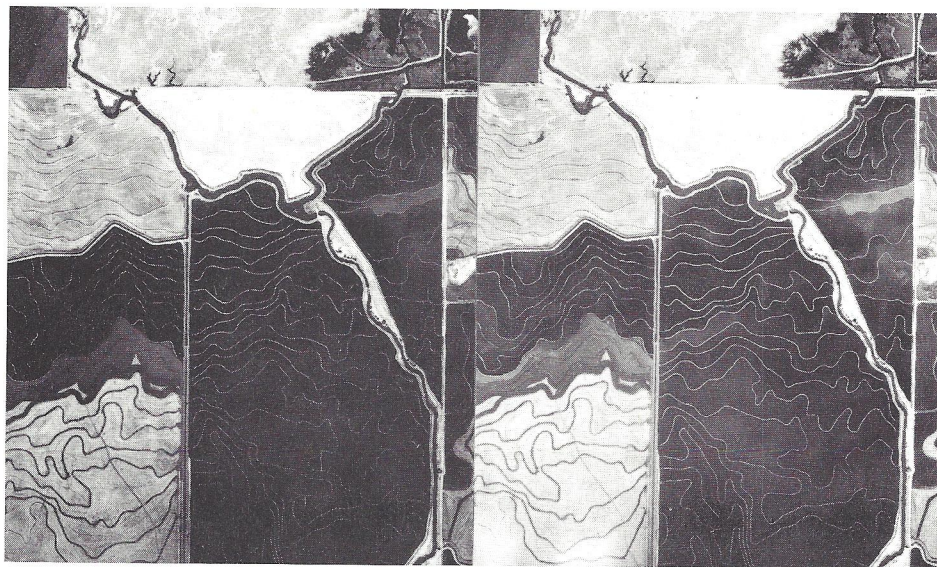
Figure 12.- Stereograms showing rice fields. Top, panchromatic film and Wratten 12 filter; bottom, infrared film and Wratten 12 filter. These fields are in California, where extreme land-use water-use economy is practiced. Dikes between fields follow the topography and form "contour" maps; this is vividly seen in stereo. Photography by Clair A. Hill and Associates, Redding, California, May 6, 1962. Scale 1:24,000.
