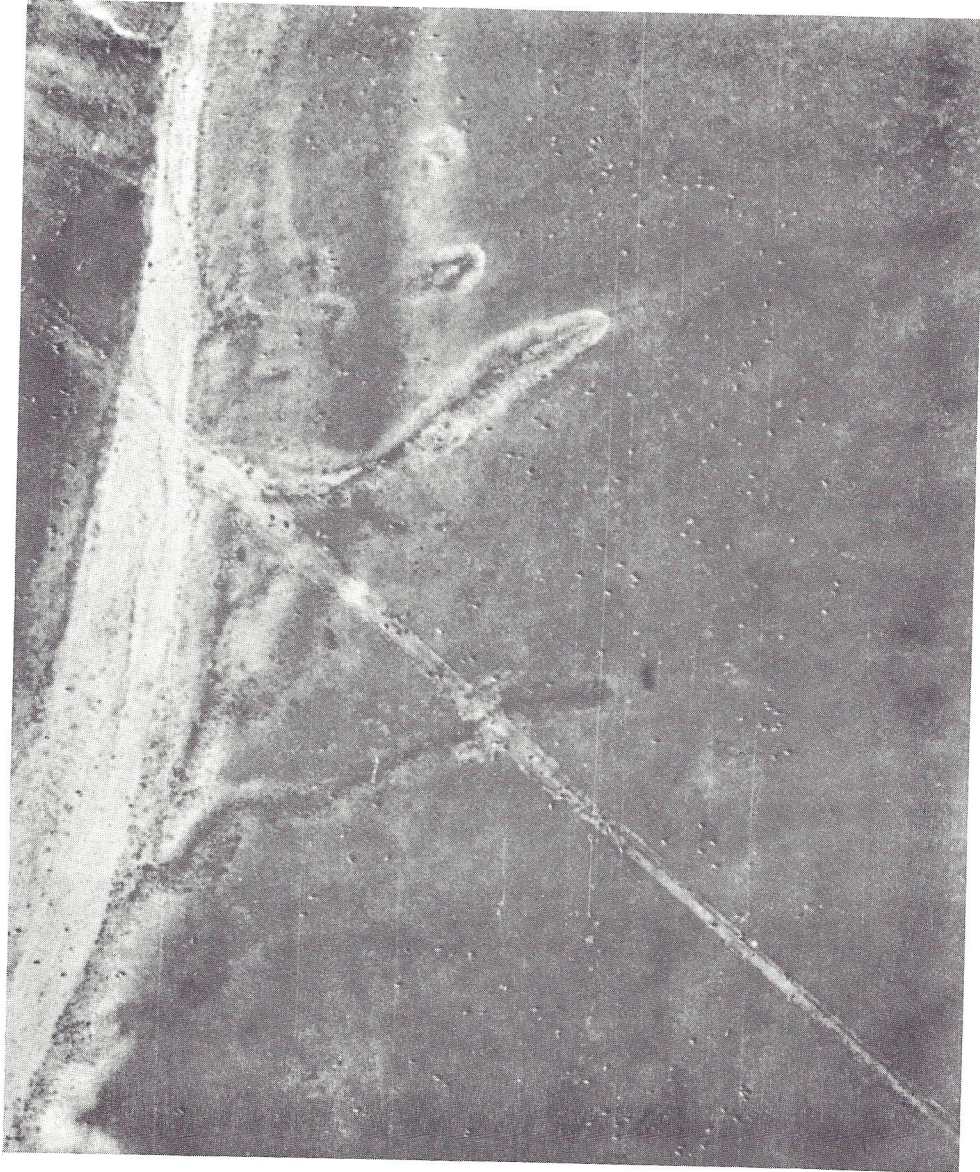
Figure 15.- Portion of exposure 354, pass 10, enlarged ten times, showing flock of sheep against grass background. Note visibility of animals even in wash. Images of lambs are small but detectable.
