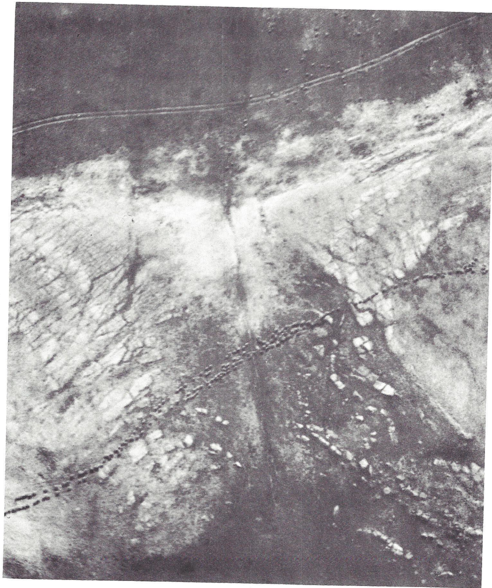
Figure 16.- Portion of exposure 296, pass 9, enlarged ten times, showing flock of sheep crossing rock outcrop. Animals are easily visible against both rock and grass backgrounds. Note round oval of bodies, light gray tone of wool.
