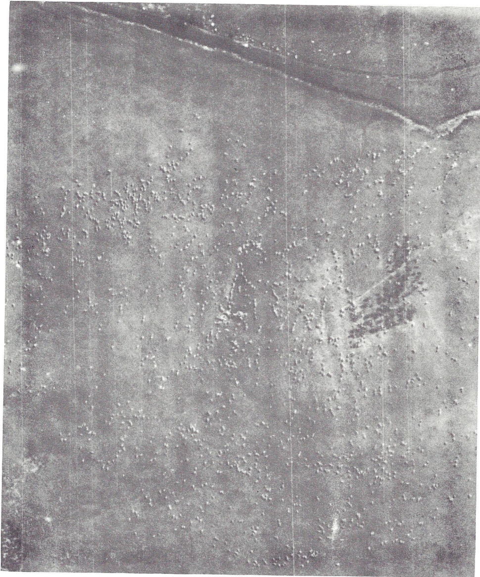
Figure 3.- Portion of exposure 343, pass 10, enlarged ten times. Contract scale about 1:13,000. This photograph represents the limiting case for the success of an operational livestock survey: detection of sheep and lambs at minimum photo scale. Images are small, but contrast and resolution are good and animals are detectable. Accurate lamb count is difficult, but possible.
